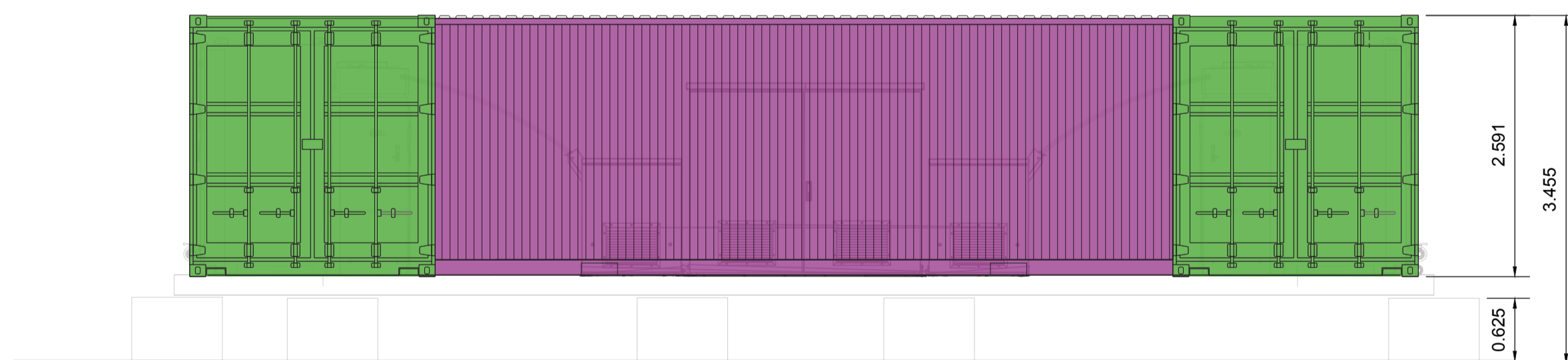
Y-Y: SECTION BATTERY UNIT ARRANGEMENT (1:50)
