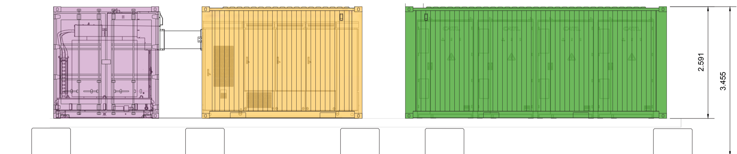
Z-Z: SECTION BATTERY UNIT ARRANGEMENT (1:50)
